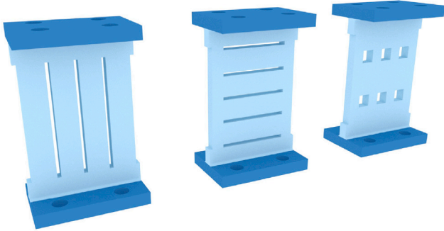
Fig. 6. Examples of slotted damper.
